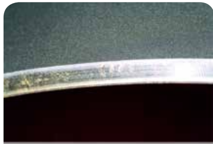
Sharp pipe bevel after blasting
