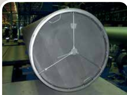
Blasting Plug in pipe after blasting
